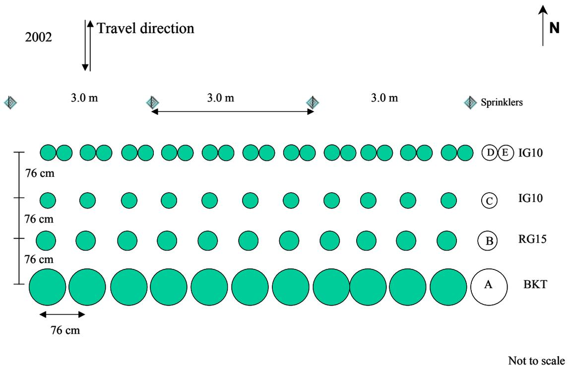
Figure 4. Set up of catch devices used in the 2002A and 2002B, KSU tests.
