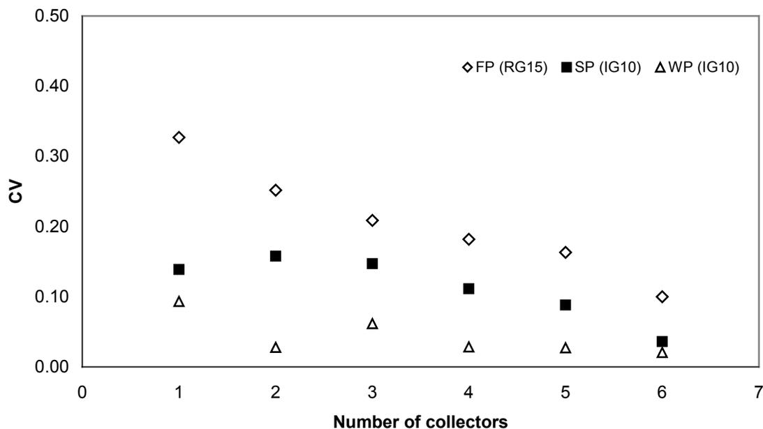
Figure 5. Effect of number of RG15 and IG10 collectors on coefficient of variability (cv) of irrigation depth under the FP, SP, and WP type irrigation packages.
